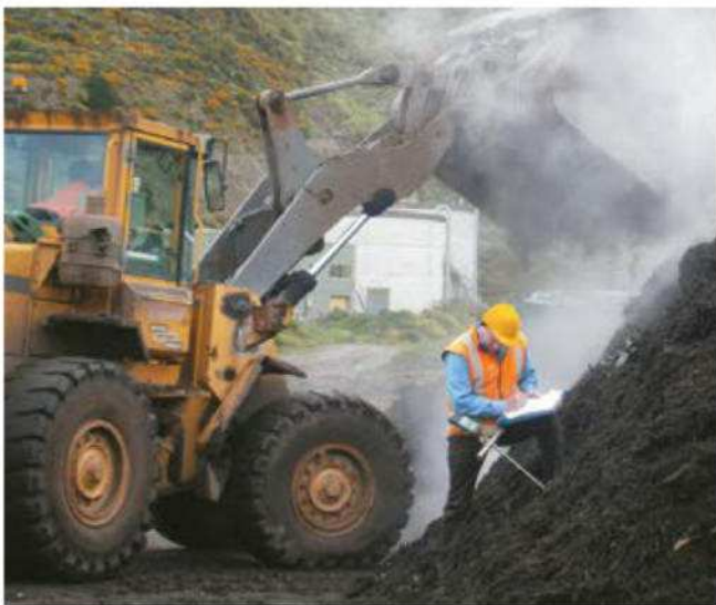
Above: Darren Hoskins, Wellington City Council's operations manager landfills, records the temperature of a compost windrow at Capital Compost.
